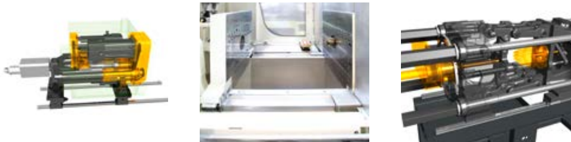
From left to right: Completely greaseless clamping unit due to covered guides on the ENGEL victory | encapsulated drive axes on an injection unit | encapsulated clamping unit on an ENGEL e-motion 100 T
