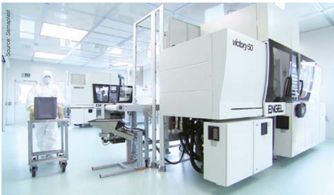
From left to right: Completely greaseless clamping unit due to covered guides on the ENGEL victory | encapsulated drive axes on an injection unit | encapsulated clamping unit on an ENGEL e-motion 100 T
