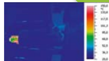
The thermal camera image shows it quite clearly: the patented GMP barrel extraction unit significantly reduces heat emission into the clean room.
