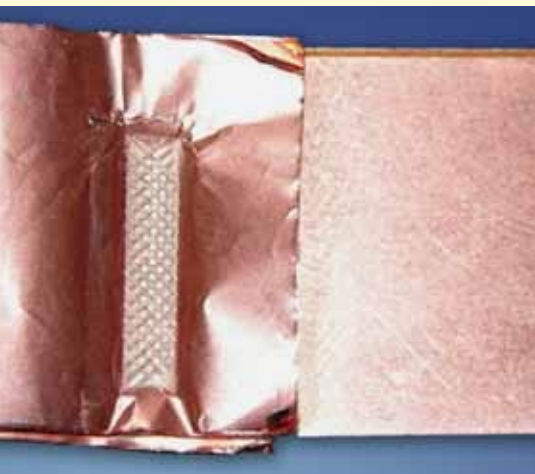
The Dual Head Ultrasonic Metal Spot Welder confidently welds up to 80 layers of foils in a single pulse.
