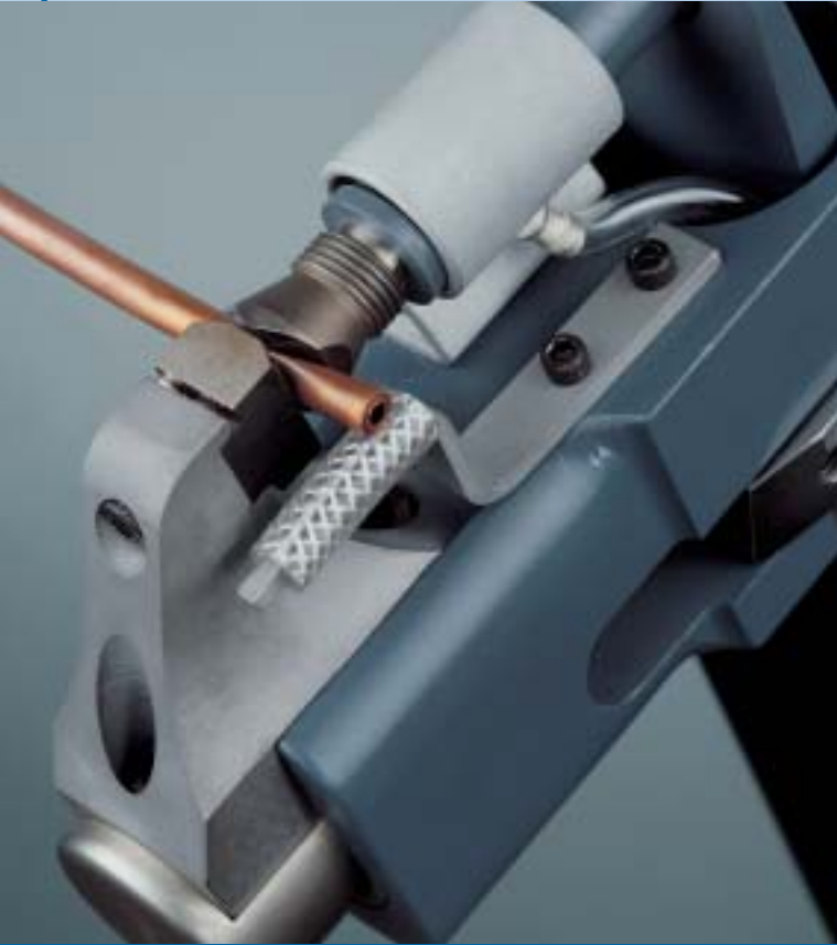
Ultrasonic Tube Terminator crimps and seals without brazing
