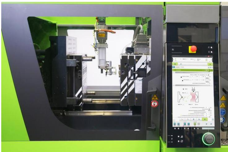
iQ motion control works with automatically optimised track planning, reducing both the teach-in overhead and the cycle time.
