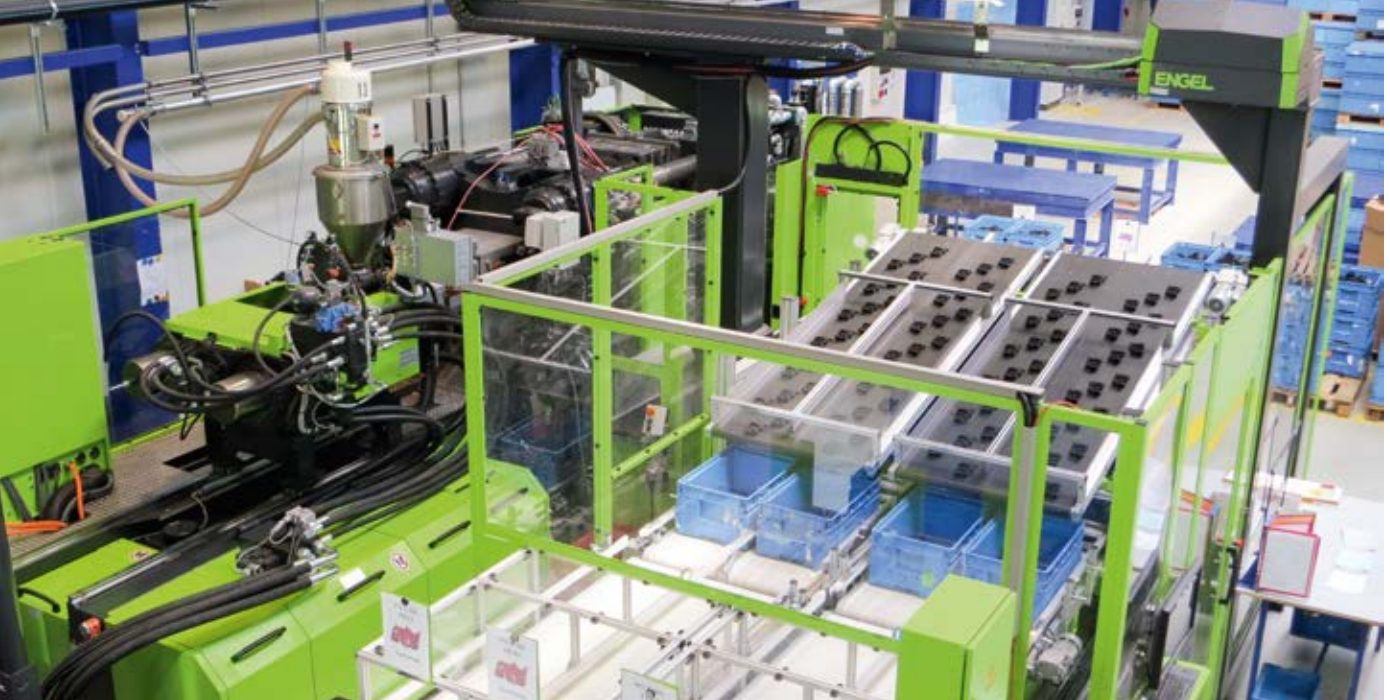
As general contractor ENGEL supplied the injection moulding machine, process technology and automation.
