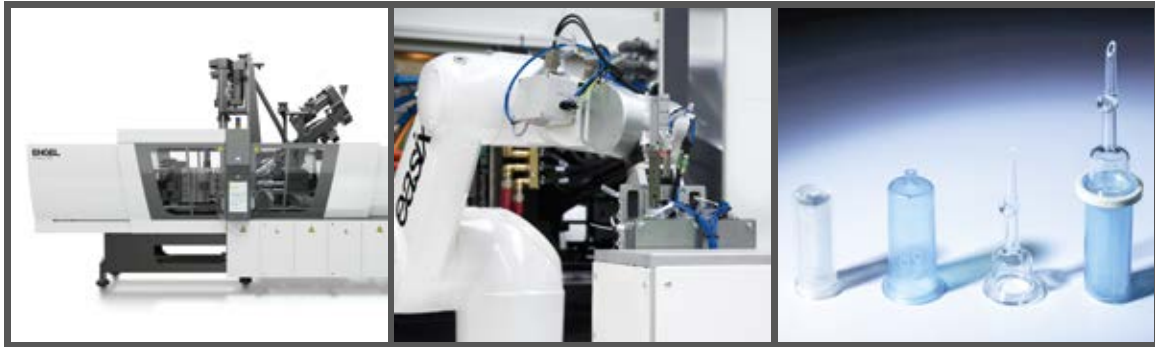
The drip chambers consist of a total of four components: a rigid upper part with piercing spike (ABS), a softer lower part (PP), a filter, and a ring, inseparably connecting the upper and lower parts (PP).
