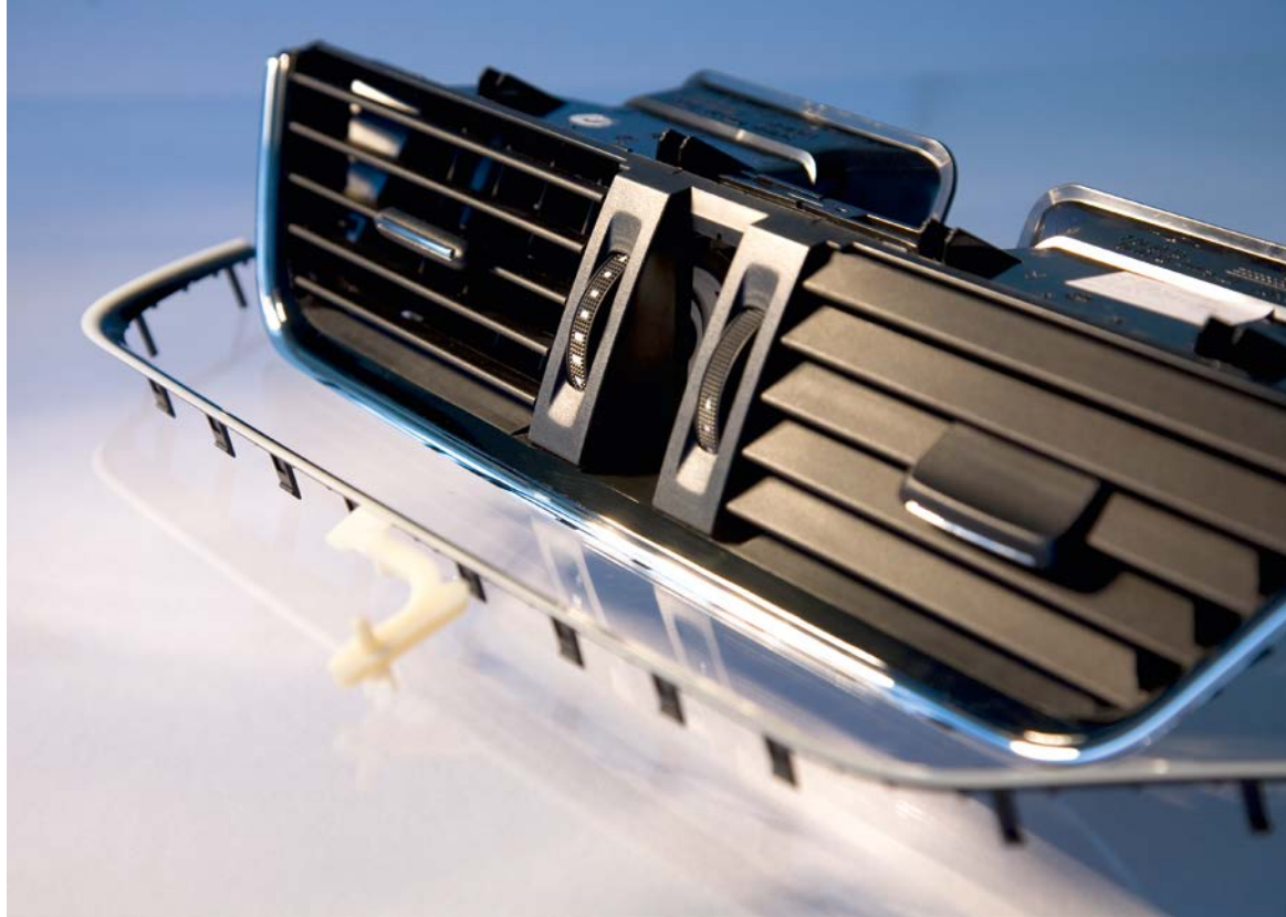
The interior of the new Škoda Octavia gleams with piano lacquer and chrome. NIFCO-KTS uses an ENGEL victory machine to produce streamlined trims for air vent panels via two-component injection moulding.
