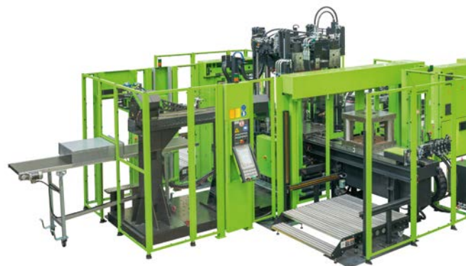
The ENGEL v-duo is more compact and more easily accessible than the conventional presses used for composite applications.
