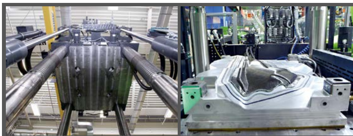
The ENGEL v-duo is more compact and more easily accessible than the conventional presses used for composite applications.
