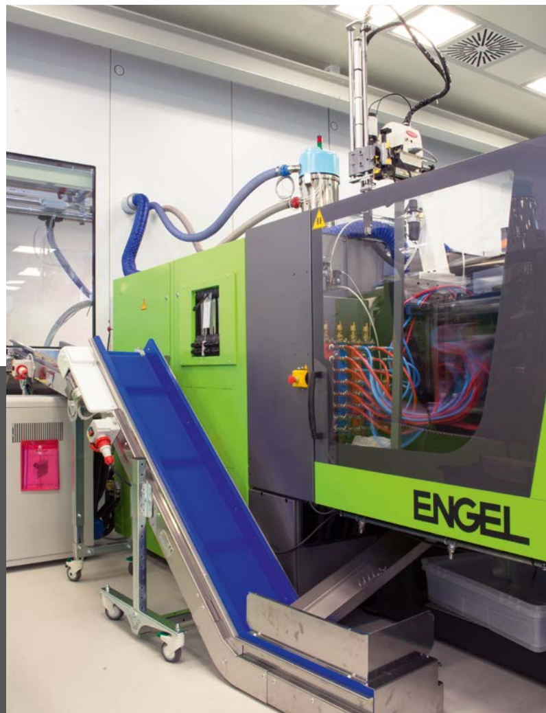
The granules come through the wall. Conversely, the sprues are transported out of the clean room through a pass box and processed in closed systems.
