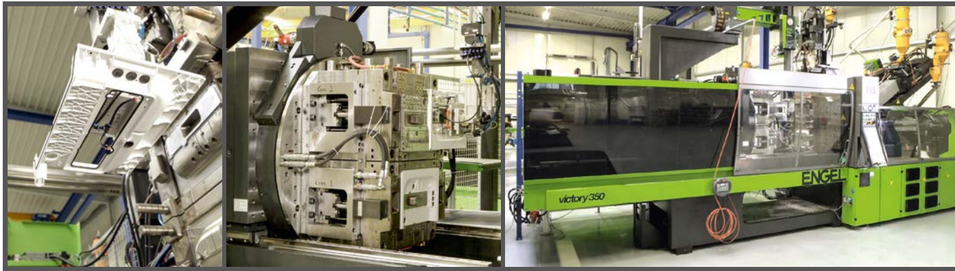
The integrated ENGEL viper robot removes finished parts from the mould.
