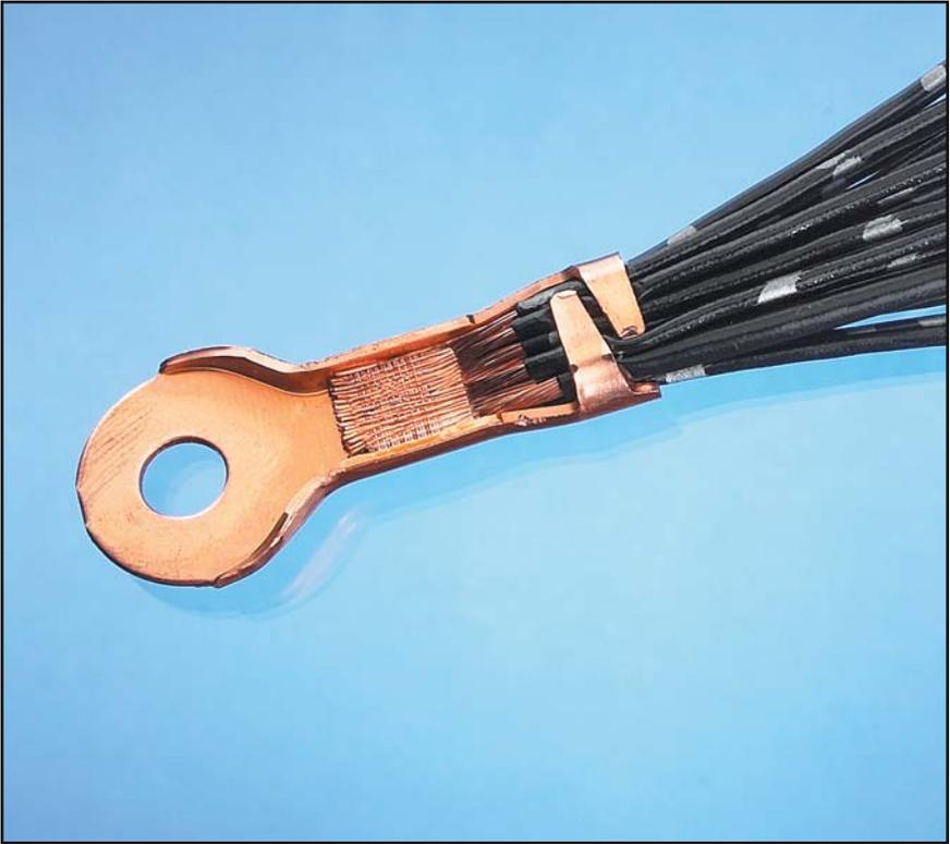
**Stranded Wire Ultrasonically Bonded to a Terminal**
