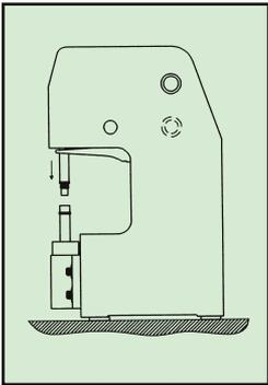
and perpendicular to the clamping force. Weld time varies according to the thickness and composition of the material to be joined and the power of the welding machine, but most spot welds can be accomplished in less than 1.5 seconds.
